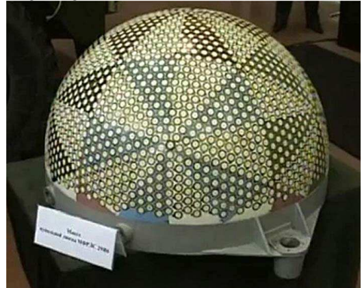
Fig. 1. Example of multisegment conformal array
